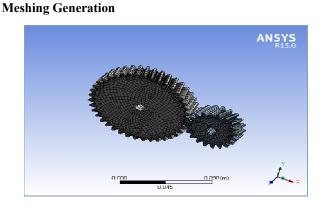
Figure 2. Meshing of Helical Gear OPair
