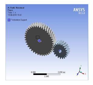
**Figure 3. Frictionless Support**
