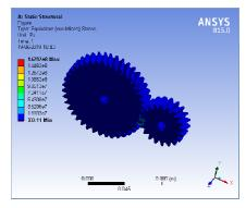
Figure 8. Equivalent Stress
